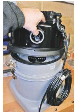
▲ The additional Hepa filter is optional to gain M class filtration levels
